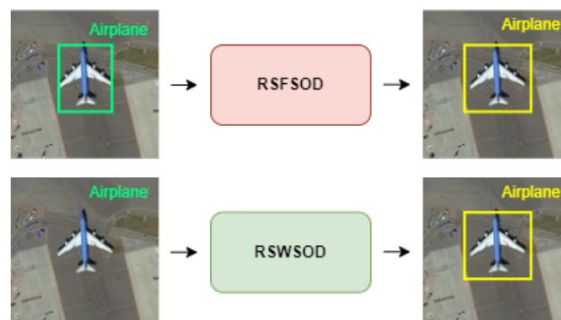
Figure 4. Visual explanation of RSFSOD and RSWSOD. In the top image, the green BB represents the ground-truth location information as given to the fully supervised detector. Such information is not present during the training of a weakly supervised detector, as shown in the bottom image.
